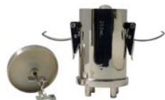
Drum Shell opened to show Agitator Blade
